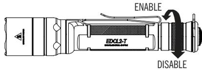
To **lock out tailcap**, rotate counterclockwise until light will not activate when pushbutton is pressed.
